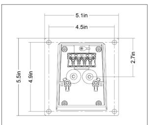
The installer must ensure to use proper means; rawplugs, screws, and expansion bolts (Not provided) to secure the luminaire to the wall material.
